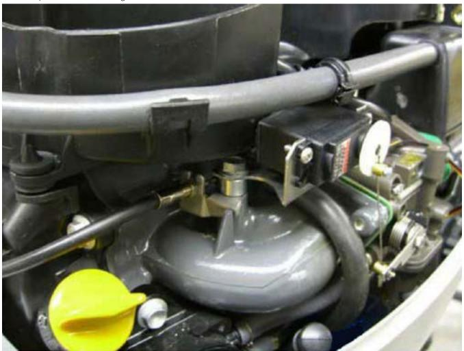
If you are working on a motor that has remote shift and throttle, there is a plastic plug in the intake manifold where the bolt goes. Use the self-tapping screw supplied in the hardware kit. Place the two spacers provided under the mounting bracket arm.
