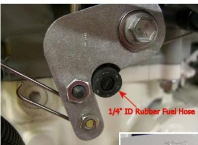
9. Using a #6 metric Allen wrench, loosen these bolts a sufficient amount to allow the servo mount bracket to slide between the bolt head and the flat washer.
